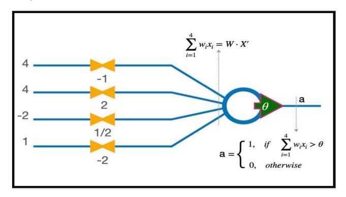
Consider the unit represented in the figure, with its input and weight distribution, step function activation, and a threshold  $\theta$  = 2.
